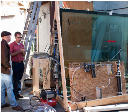
Figure 6 This configuration simulates a worst case scenario for an open system operating in the air displacement mode, with positive external pressure such that the mixing rate of humid air infiltration and dry air controls the cavity condition. Since relative humidity and saturation pressure are strong functions of temperature, the outer surface of the glazing is cooled in some tests to produce a temperature field that corresponds to winter conditions. The actual test piece and cold chamber utilized to produce this effect is depicted to the right.
