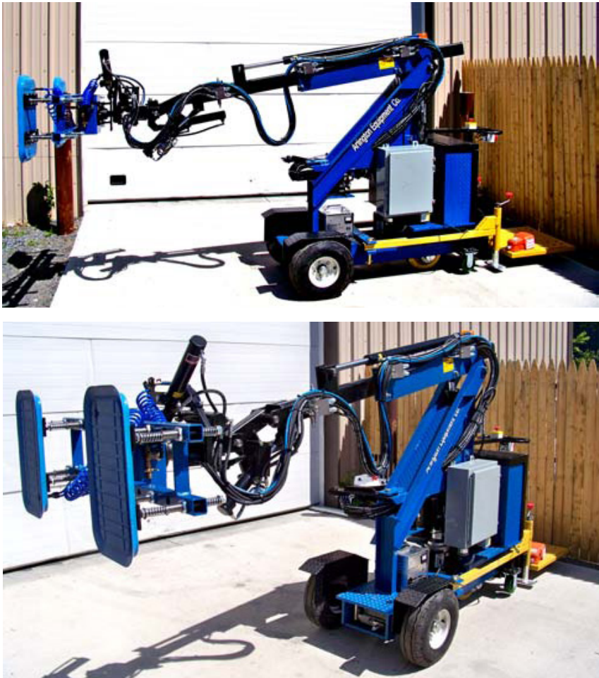
Figure 5: A mobile glass manipulator is of the mobile category, designed for field installation of large glass lites. This mobile glass manipulator can be purchased as shown; however, they are often customized to achieve the project’s requirements. This particular model can manipulate a 2,000lb piece of glass 6’ horizontally from the front of the machine’s wheels. These manipulators are often used if 2-3 men cannot handle a lite safely, there is limited access and clearance to install a lite, or just for the sake of production. They are also designed to fit through a standard doorway (3’ x 6’-8”) and fit into an elevator.
