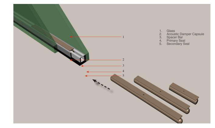
Figure 2. Components of the acoustically enhanced insulated glass unit
