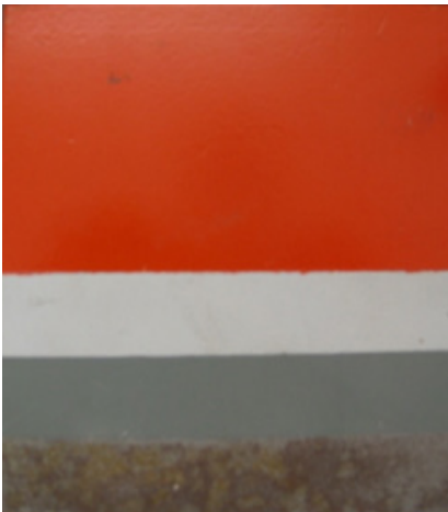
Figure 6. Steel finish sample showing cut back layers starting with raw steel (Bottom), 1st layer primer, 2nd layer primer, finish coat (Top). Also an example of how to apply step back paint process for field welding and later paint blending.
