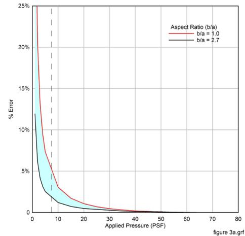
Figure 4. Error between the numerical simulation and the empirical equation for SS plate.
