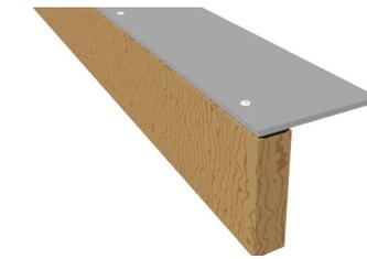
Figure 6a. Flat Edge Condition; lay a 1-inch wide neoprene gasket (1/8" thick) along the four sides of the box. Secure the panel using 3/8" stainless steel self-taping screws on the corners and on 12" centers along the edges.
