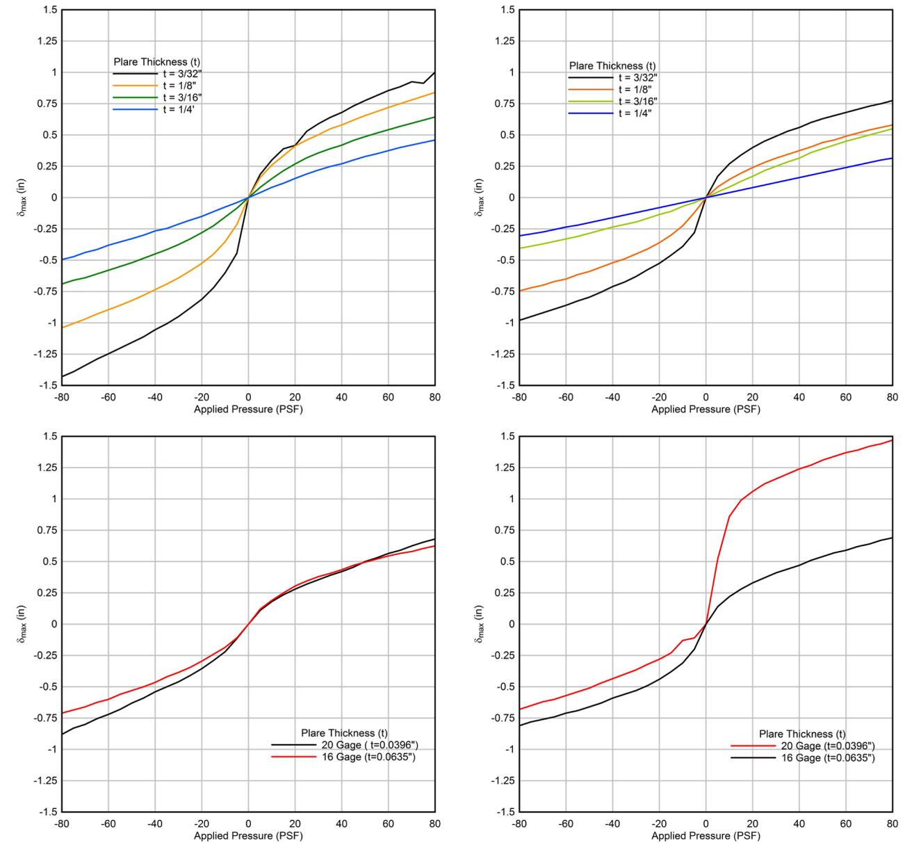
Figure 7. Plot of deflected shapes or various material and boundary conditions. (Top-Left), Silicone sealed flat aluminum plate, (Top Right) Flat-fixed screws with aluminum plates, (Bottom-Left) 4-sided folded fastened galvanized sheet metal, (Bottom-Right) 2-sided folded fastened galvanized sheet metal
