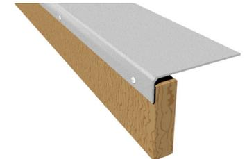
Figure 6b. Bent edge condition; use a bent edge of 1-1/2" on two or four sides of the panels (if using bent edge on only two sides, apply to the long sides). The bent radius is not to be less than two times the thickness of the material. Lay a 1-inch wide neoprene gasket (1/8" thick) along the four sides of the box. Secure the panel using 3/8" stainless steel self-taping screws on the corners and on 12" on center along the edges
