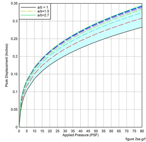
Figure 2. Effect of the plate aspect ratio on peak plate deflection.
