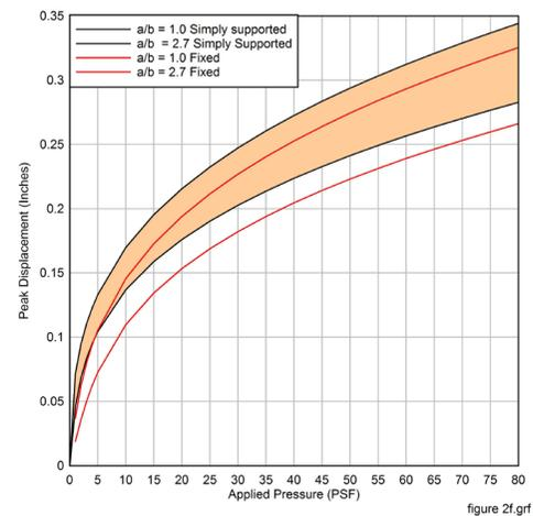
Figure 3. Effect of the plate support condition on the peak plate deflection.
