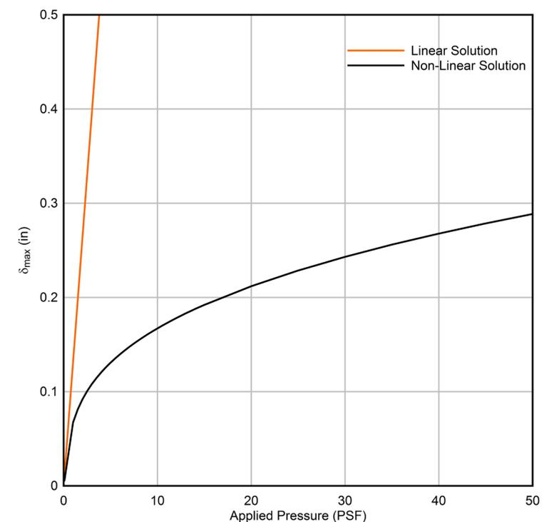
Figure 1. Peak displacement of a rectangular panel (3'-0" W x 5'-0"H), with a thickness of 3/32". The linear solution (show in orange) could significantly over estimate the peak displacement of the panel.
