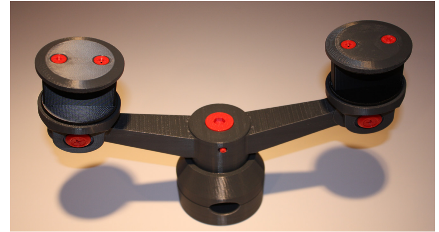
Figure 3: 500 Fifth Avenue Atrium Wall cable fitting prototype.
