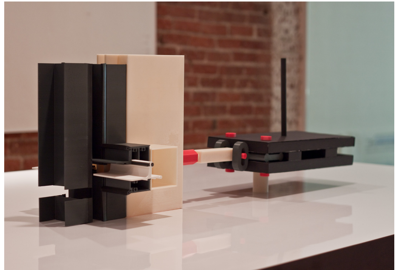
Figure 4: Nashville Music City Center facade system with aluminum cassettes (front) attached to aluminum frame, braced back to horizontal steel truss (black) suspended by vertical rods.
